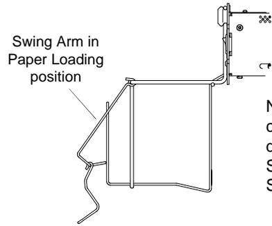
**NOTE:** Do NOT close the printer door while the Swing Arm is in the Stacking position.
